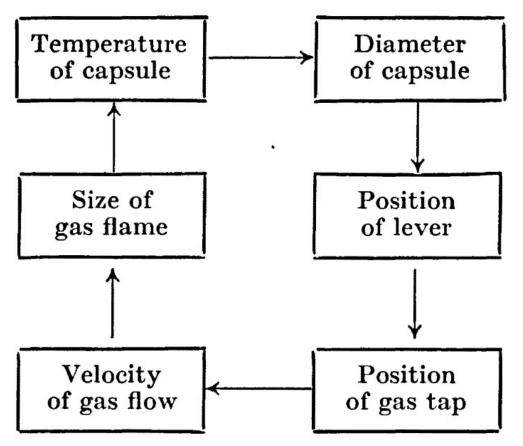
The reader should verify that each arrow represents a physical action which can be demonstrated if all variables other than the pair are kept constant.<sup>6</sup>
