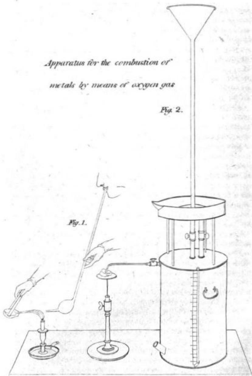
*Fig. 1. Ionizing charcoal with a taper & blow-pipe. Fig. 2. Combustion of metals
