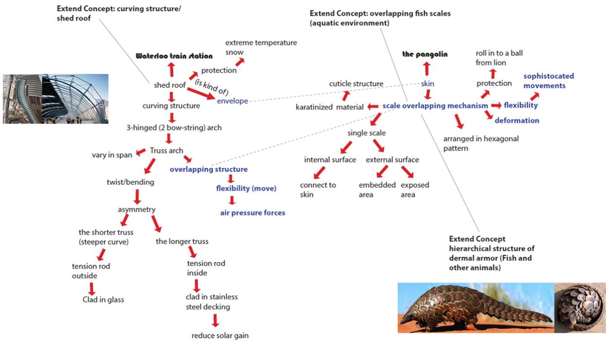
Figure 5. The concept map analyzes London's Waterloo Station roof design, showing biomimetic influences from pangolin and fish scales. The diagram connects structural elements (curved trusses, overlapping glass panels) with biological principles (protection, flexibility, load distribution). Red arrows illustrate relationships between natural scale mechanisms and architectural implementations, demonstrating how animal armor patterns inspired the station's distinctive overlapping glass structure.
