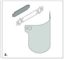
Visor component comes in two sizes. Use white silicone for small visors. Use red silicone for large visors.
